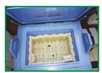
Cold box packed with icepacks and having a thermometer
